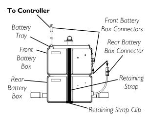
FIGURE 11.3 Removing/Installing the Battery Boxes
